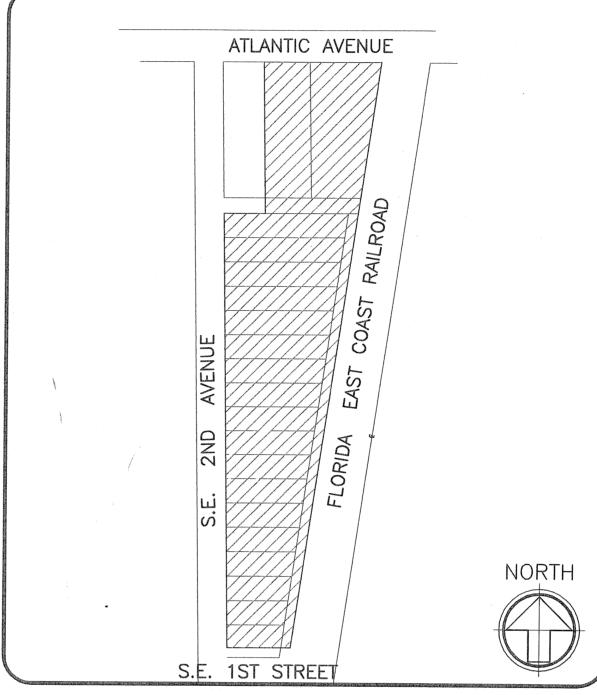
BEARINGS SHOWN HEREON ARE BASED ON THE WEST LINE OF BLOCK 86 AND THE EAST RIGHT-OF-WAY LINE OF FLORIDA EAST COAST RAILWAY. SAID MONUMENTED LINE BEARS NORTH 08°27'37"
